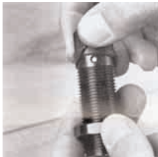
Push the rubber seal ring up to expose the fill hole.
